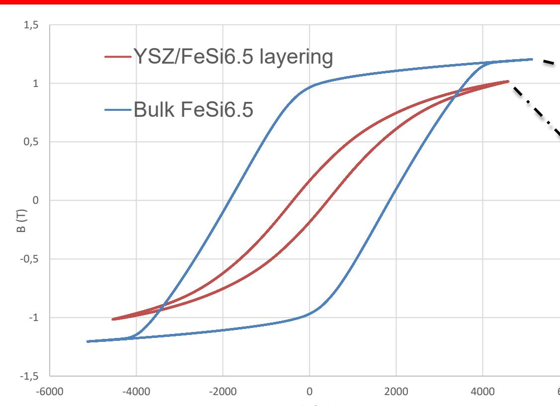
Hysteresis loops at 50 Hz after heat treatment ( $T = 1150^\circ C$  for 2 h 30 min under hydrogen atmosphere) for a Fe-6.5%Si alloy and a FeSi6.5/ceramic multi-material toroid
