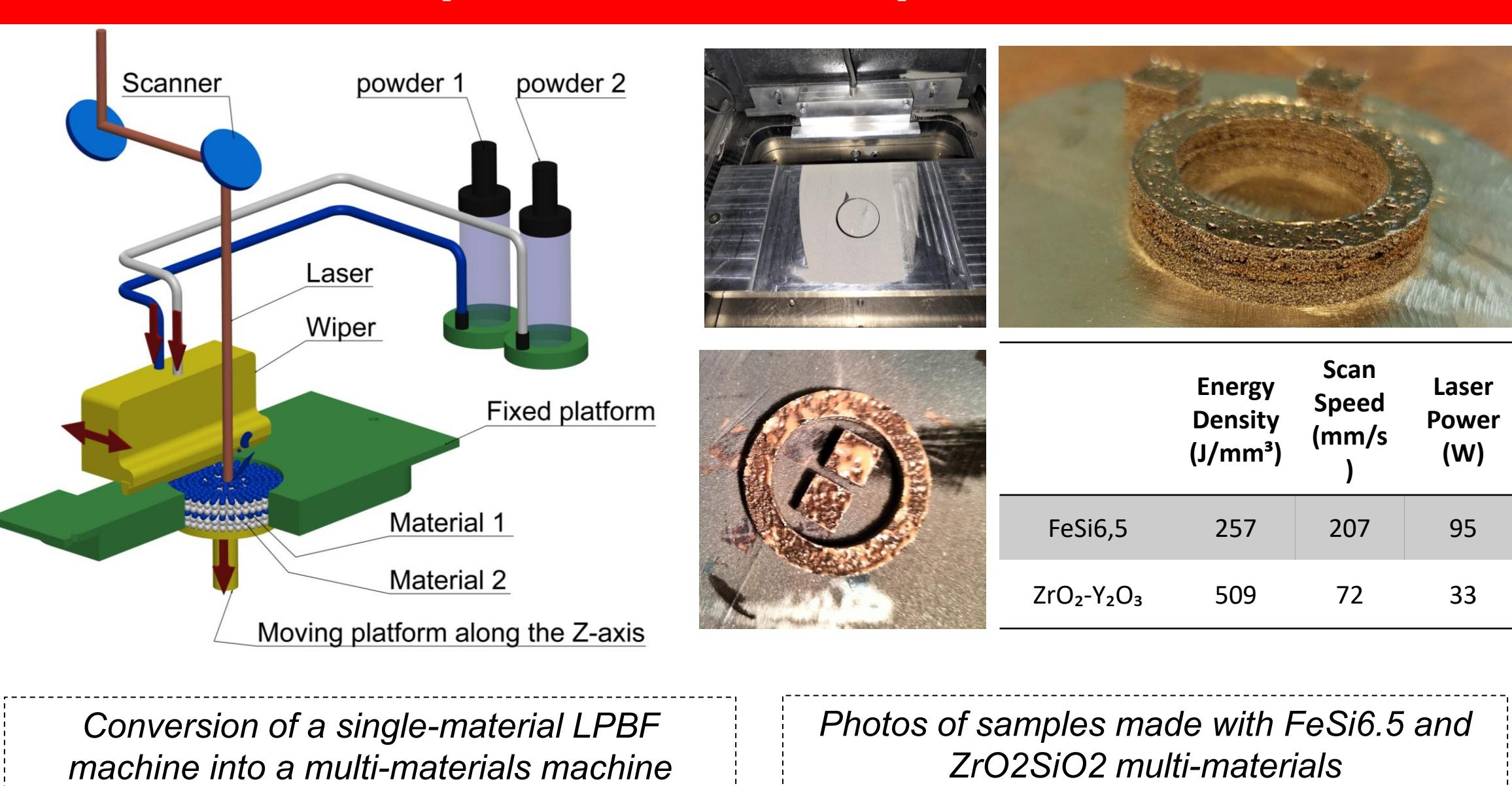
Conversion of a single-material LPBF machine into a multi-materials machine
