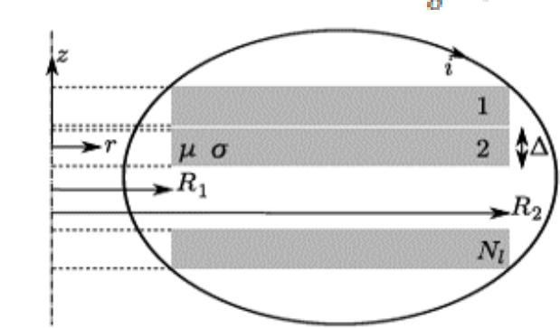
Numerical model for estimating magnetic losses in a solid material and in a laminated sheet stack [Miroslav Markovic, 2009]
