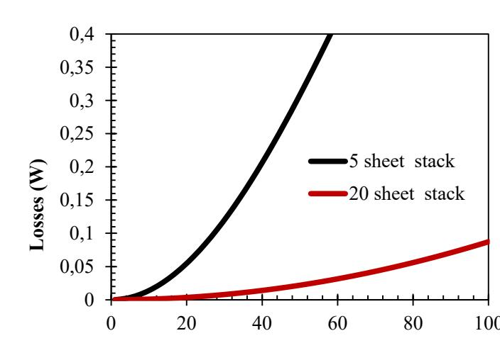
Comparison of magnetic losses between a 5-sheet laminate and a 20-sheet laminate with the same overall thickness. [Miroslav Markovic, 2009]
